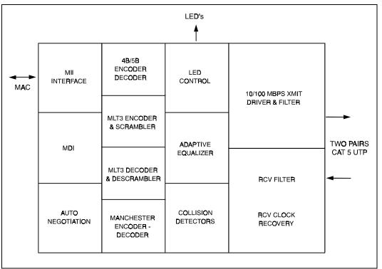
Figure 2. 82555 Simplified Block Diagram
